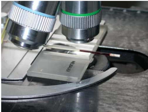
Figure 23 a – WOO's test: direct examination of the buffy coat through the capillary tube
